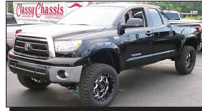
Toyota Shown With 6" Lift Kit, Custom Wheels & Tires & Painted To Match Pocket Fender Flares
